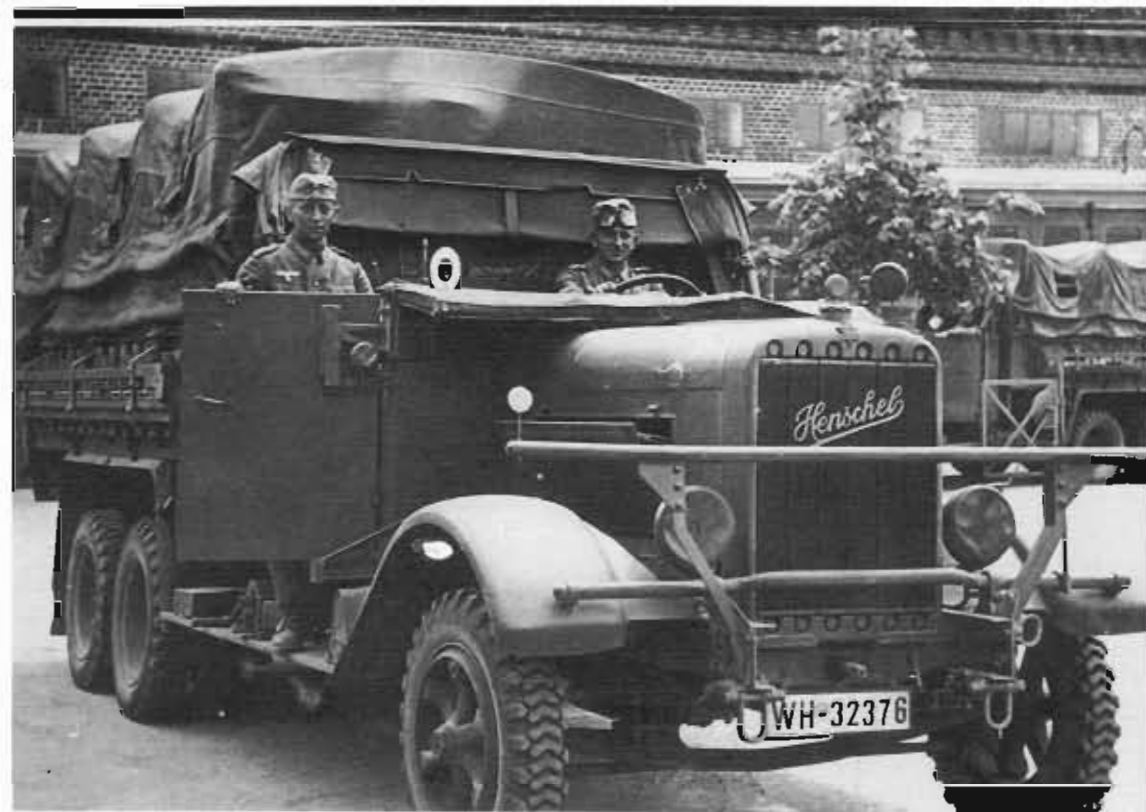
A Henschel Type 33 from the Berlin district. All of the lights have camouflage covers – a camouflage light has not yet been installed. Note the eye of the winch cable under the left headlight; it ran through the fender (flap on the back).
