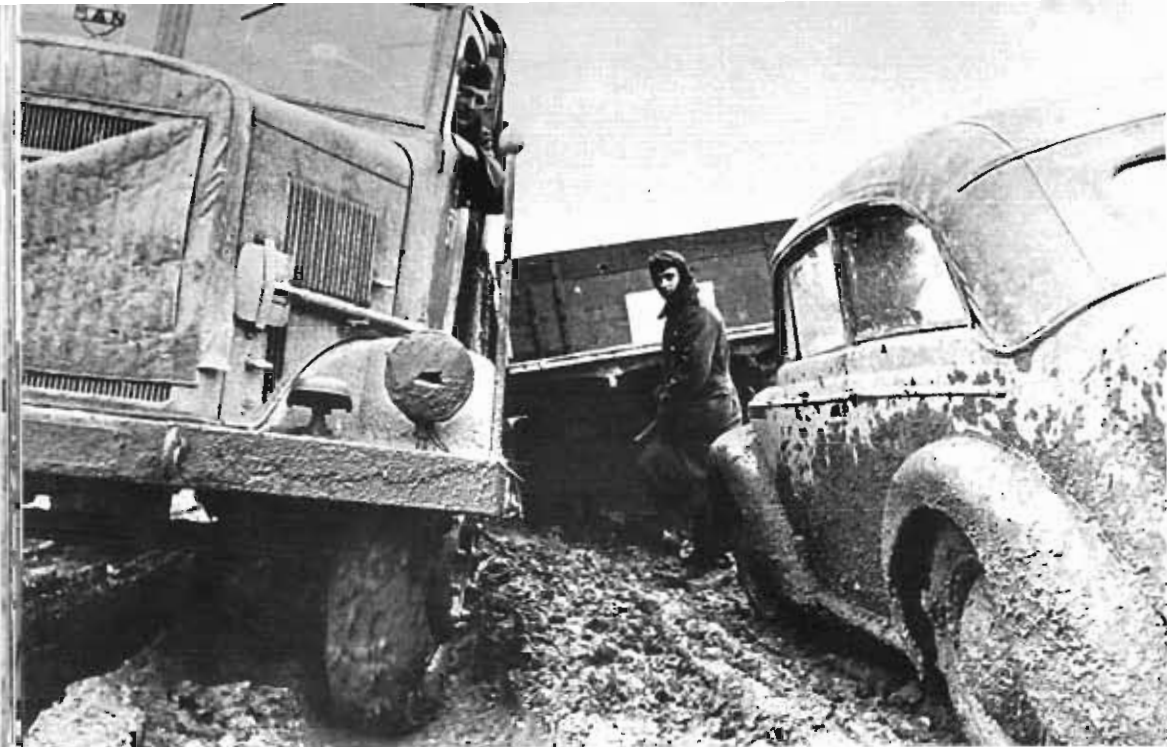
This MAN Type ML 4500 S fights its way through the mud (4/28/1942). The S version is recognizable by the lack of reduction gears (in front), the depression in the middle of the front wheel, and the louvers of different lengths, which can be seen here under the spade. (BA)
