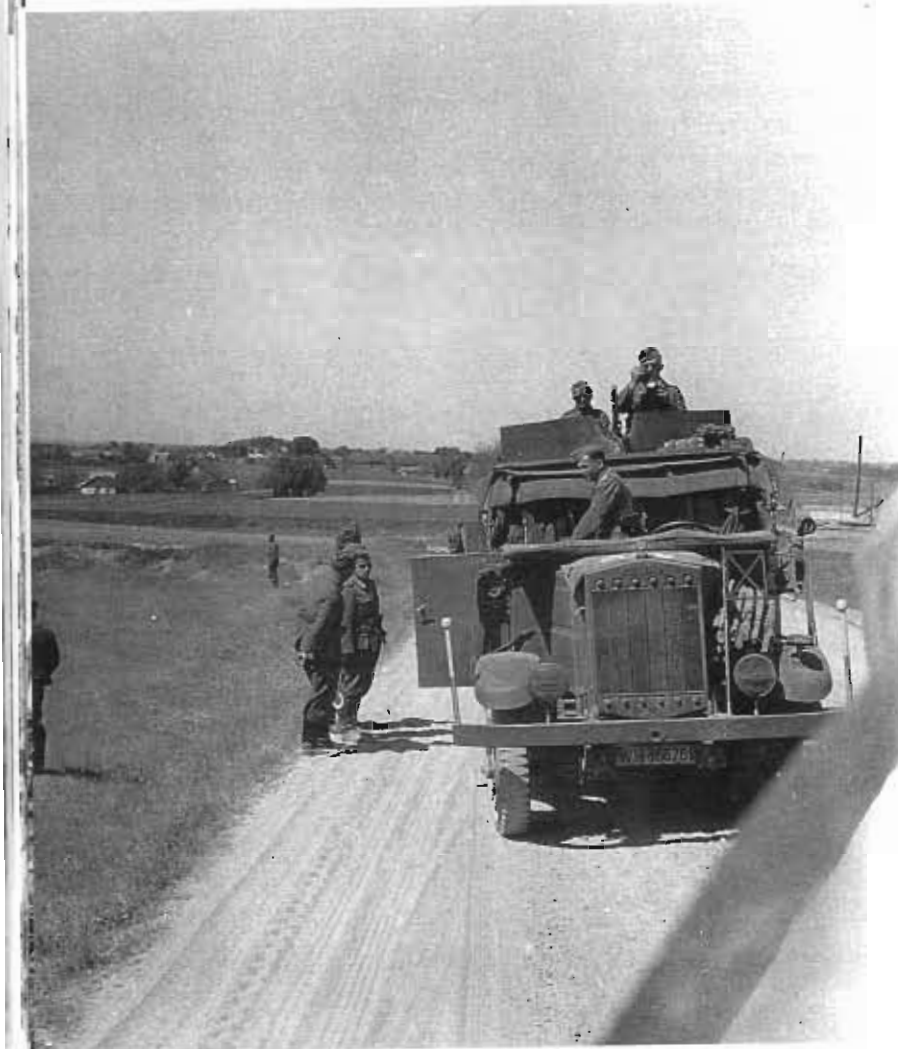
"Medium off-road Lkw. (o) Krupp L 3 H 163" of the 5th SS Panzer Division "Viking" on the Danube bridge at Nikopol, Bulgaria. The 3-ton (6 x 4) truck had a 6-cylinder, 7.5-liter gasoline motor producing 110 HP. (BA)
