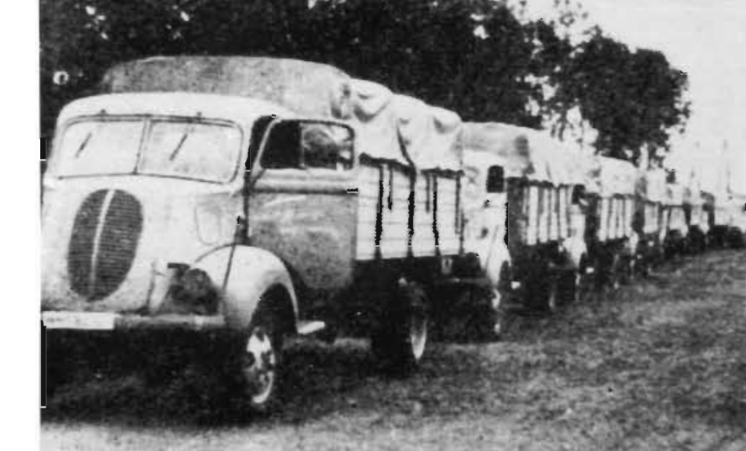
In 1943-44, small numbers of an all-wheel drive, cabover version of the 3-ton truck were built. The American Ford COE of 1939 (COE = cab over engine) was its godfather. The picture comes from "Krafthand" of January 1945 and is entitled: "Supply trucks roll in long columns from our factories to all fronts."
