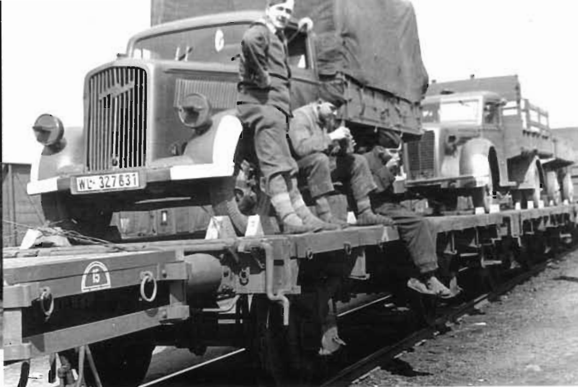
Rail transport for a 3-ton Opel Blitz S with carefully attached wheels and lashings. The "Comrades of the Luftwaffe" where comfortable slippers over their colorful service socks. Note the slits of the headlights – and the lack of a camouflage light. The second truck may be a British Commer.
