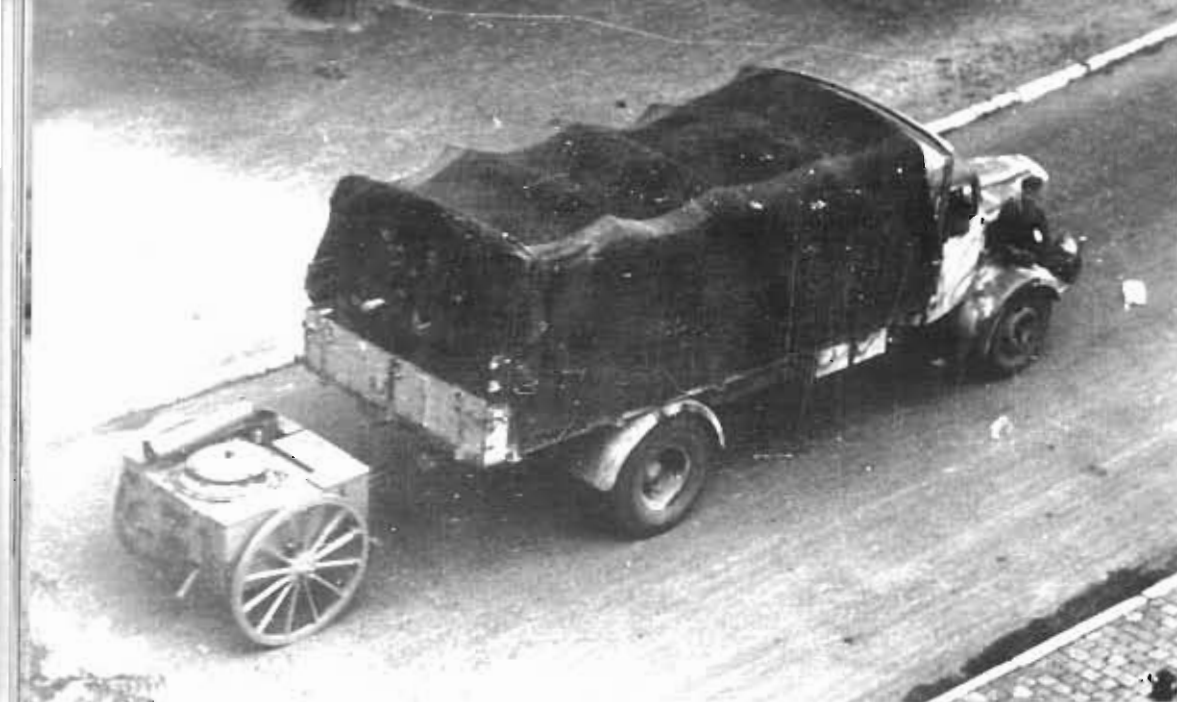
The German troops withdrawing from Brussels (Sept. 2-3, 1944) were secretly photographed by a Belgian. The truck, full of soldiers, is towing a "Large Field Kitchen Hf. 13", which was intended to be horse-drawn. The light-colored camouflage paint and the aircraft observer (Lucki-Lucki) on the front fender are easy to see. The truck is a Mercedes-Benz Type L 4500, surely the S version, as one can tell by the recessed wheel hub at the front.
