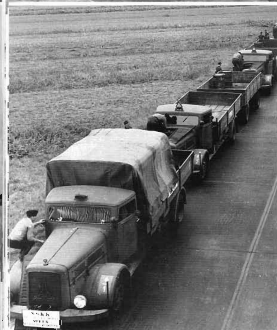
In 1941, forty Magirus L 365 6-ton trucks (with Deutz Diesel engines, 6 cylinders, 13.5 liters, 145 HP) were rebuilt into rail trucks at the Reichsbahn works in Opladen.
