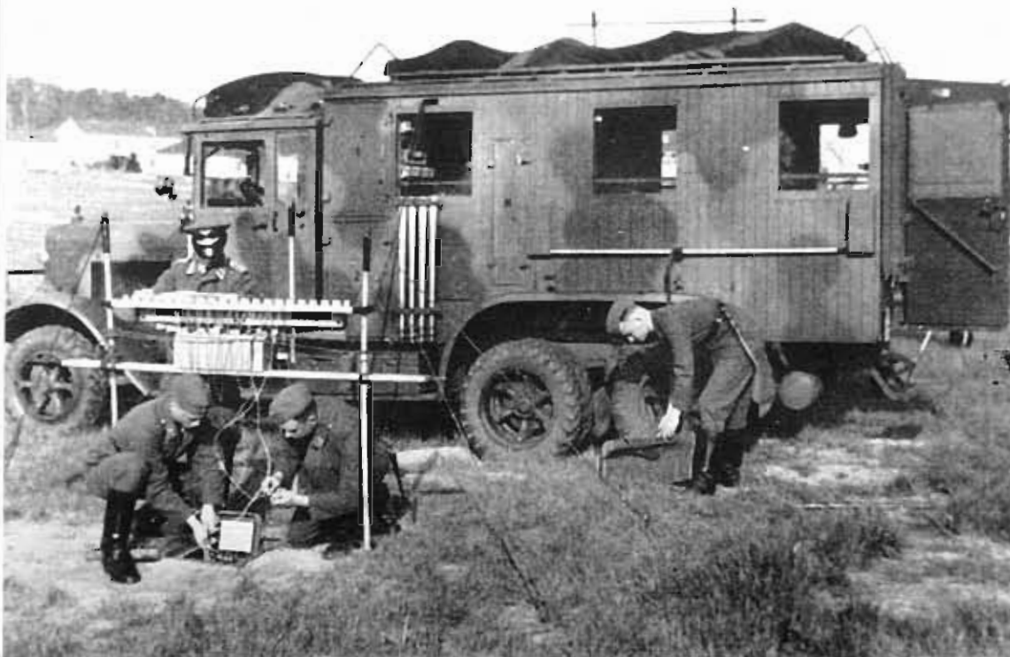
A Henschel Type 33 with closed body and cab, as a telephone service truck (Kfz. 72). The two compressed-air tanks for the brake system are easy to see under the rear.
