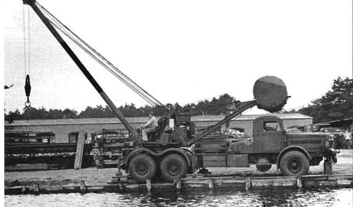
Side view of the 9-ton FAUN with a crane that could lift 5 to 8 (maximum 10) tons. The "blind axle" behind the front wheels can be seen.
