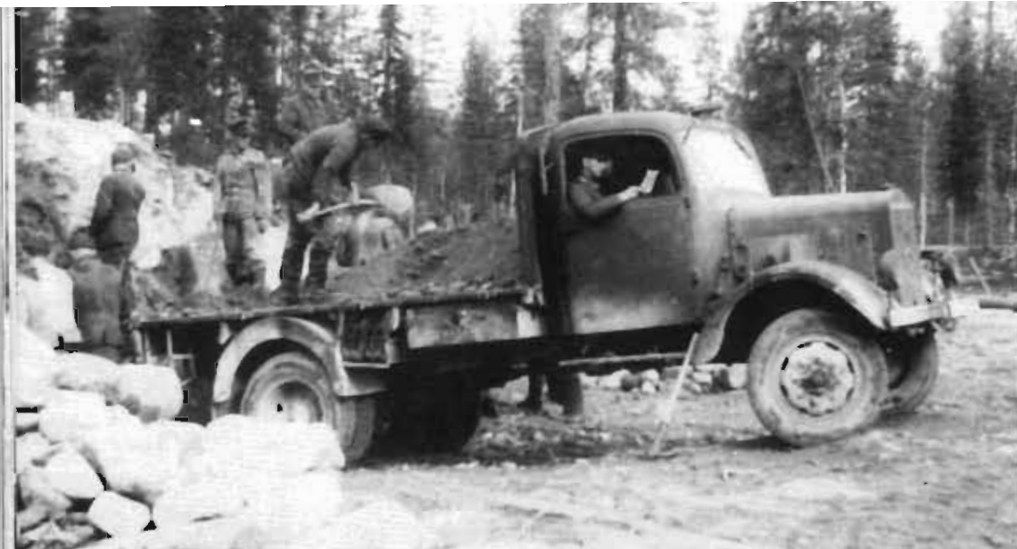
The Mercedes-Benz Type L 1500 S was built since 1937 with both 47 HP gasoline and 45 HP Diesel motors. The 1.5-ton truck was too small and uneconomical for military use. The picture shows a flatbed truck of SS Mountain Engineer Battalion 6 (Division "Nord") at the Pya Lake in northern Finland in the autumn of 1943.
