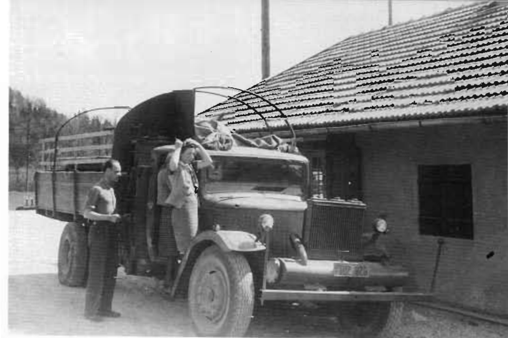
The Citroen T 45 was also produced in series with a wood-gas generator. Here such a truck is seen after the war, scrounging in Upper Bavaria (B/Y 102 929).
