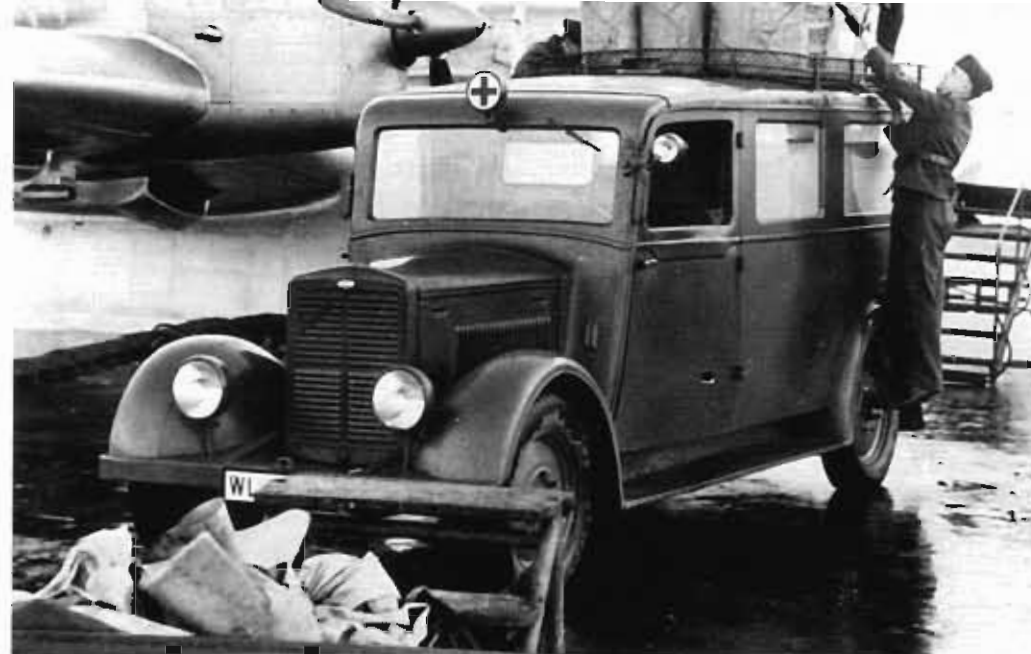
The Phänomen Granit 30 had a 55 HP motor and a load limit of 2.3 tons. Only a few examples reached the Wehrmacht. This is an ambulance (Kfz. 31) of the Luftwaffe loading medical supplies into a Do 26.
