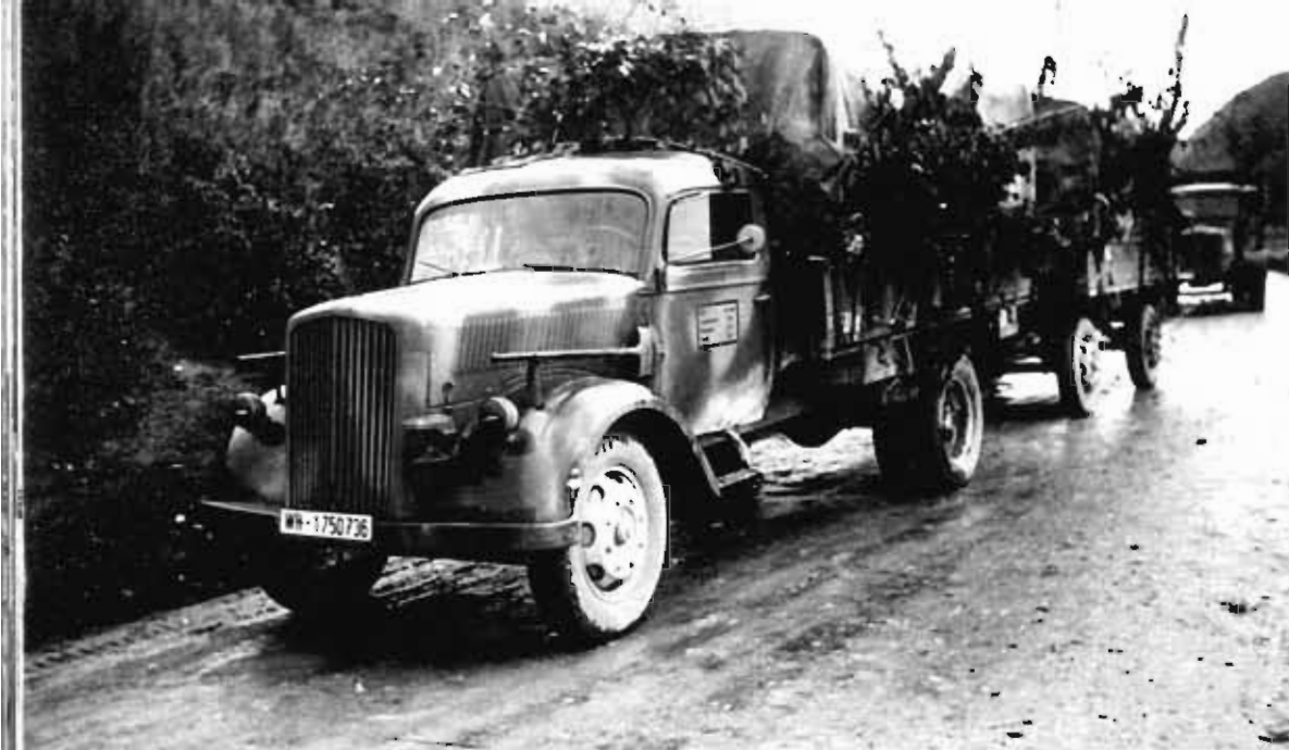
A 3-ton Opel Blitz S of Landing Engineer Battalion 86 in the Strumica-Strip area, autumn 1944. A late version with refined grille, the small headlights of the last war years, simplified steps, no rear fenders and no triangular trailer symbol.
