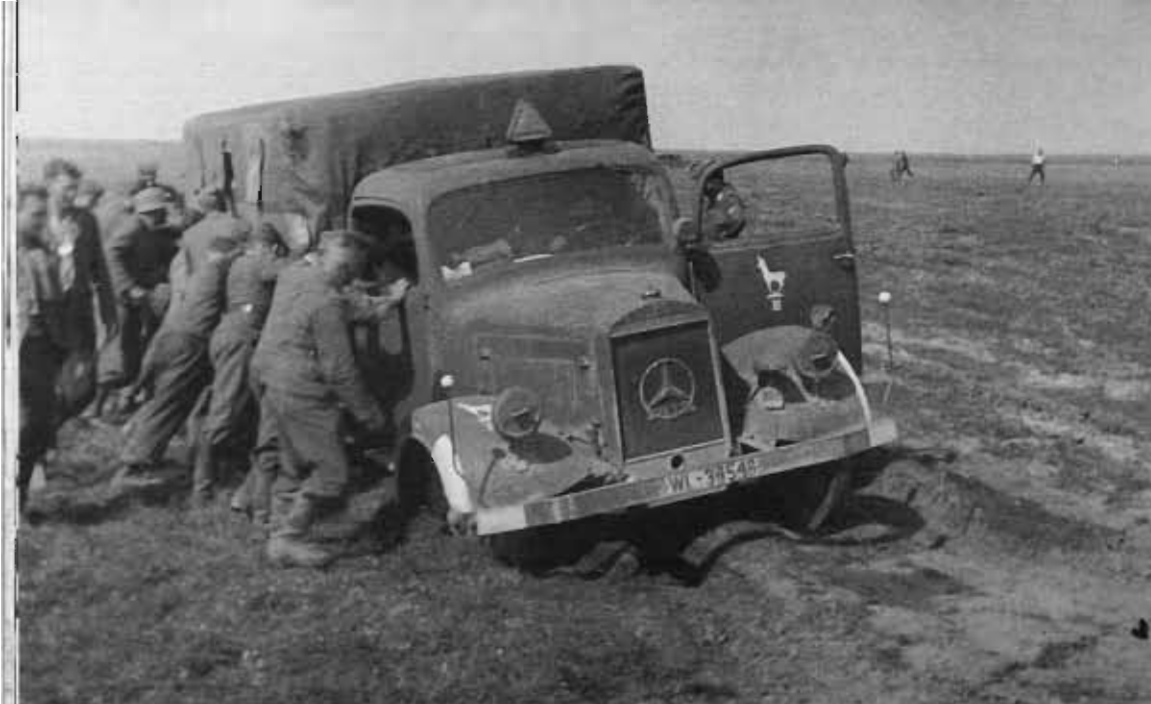
Some 16,000 of the 3-ton Mercedes-Benz Type L 3000 S (4 x 2) truck were built from 1938 to 1944. The vehicle had an OM 65/4 Diesel engine (OM = oil motor): 4 cylinders, 4.8 liters, 75 HP. This vehicle, of a Luftwaffe field hospital, got stuck on the plains of southern Russia in 1942.
