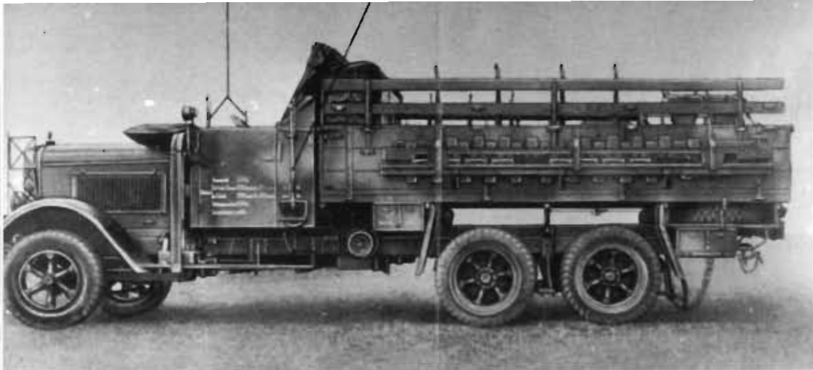
The Henschel & Son Type 33 3-ton truck as medium AA gun truck (m.gl.Lkw. off.(o)), which served as a towing vehicle for the 3.7 cm Flak 18 gun and had as its crew a driver, an aide, a gun leader, seven gunners and two air sentries. On the frame behind the cab is the 5-ton winch, over it the case for the 25-meter (sometimes 50 meter), 14 mm towing cable with 15-ton strength. The two spare wheels were attached under the bed at the rear. (a = two guns in racks, c = long spade).
