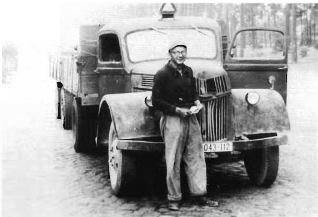
The Ford V 3000 S appeared in 1943 with a larger radiator as the G 388 TS (4 cylinders, 3.2 liters) and G 398 TS (V8, 3.9 liters). The vehicle had additional louvers at the front of the motor hood and two air intakes on top of the hood. The picture shows "one of the survivors" in Berlin shortly after the war ended.
