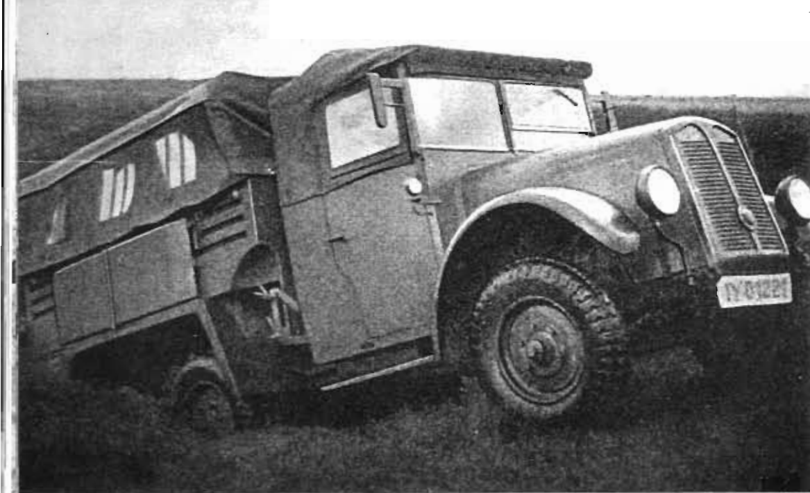
The progenitor of the 1.5-ton Krupp (6 x 4) truck was the "light off-road vehicle with air-cooled 60-HP carbureted motor (L 2 H 43) or 50-HP Diesel motor (LD 2 H 43)." Its motor hood had not yet taken on the typical sloped form.
