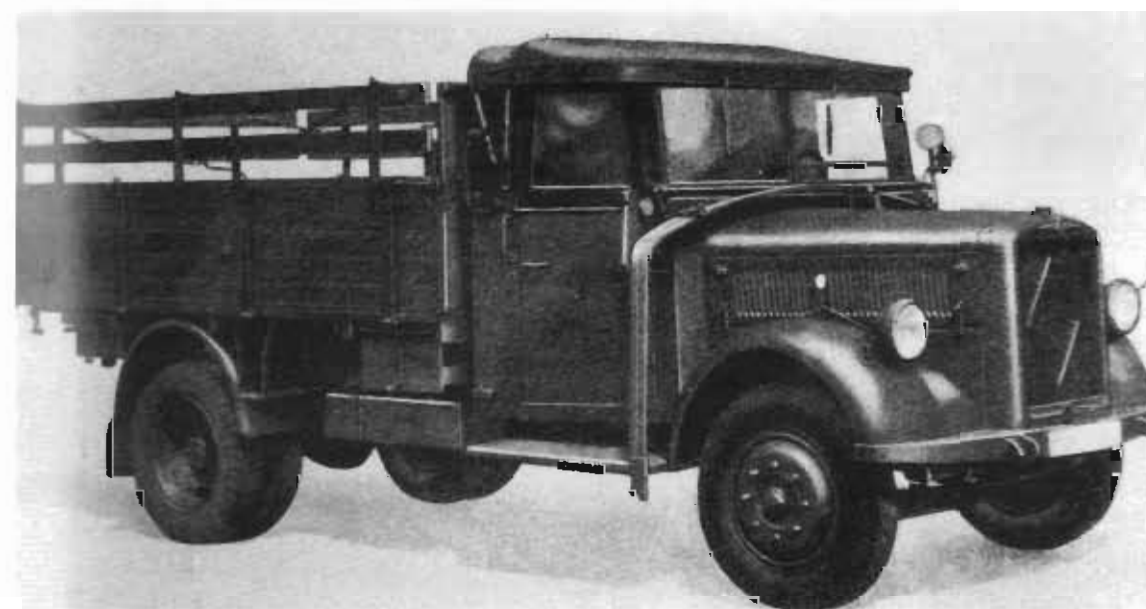
The "Lkw 3 t Borgward Type 3 t Benzin G.W.", as portrayed in D 669/35 of 9/3/1941. The vehicle was portrayed as a medium truck, open (o), and had a 6-cylinder, 3.4-liter motor that produced 73 HP. This type generally had an open uniform cab.
