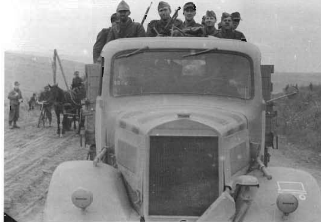
A Mercedes-Benz Type L 3000 carrying Romanian soldiers in the spring of 1944. By the attachment of the pick and shovel, this may well be the A version. Note the typical mount of the camouflage headlight and the Czech MG 26 gun. (BA)
