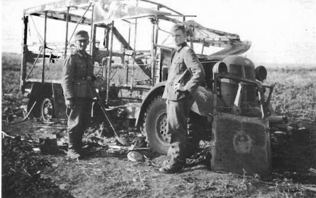
4600 of the Austin K 30 (4 tons, 4 x 2, 60 HP) were built. This is a burned-out ambulance of the 1st Mountain Division; the stretcher racks can still be seen clearly.
