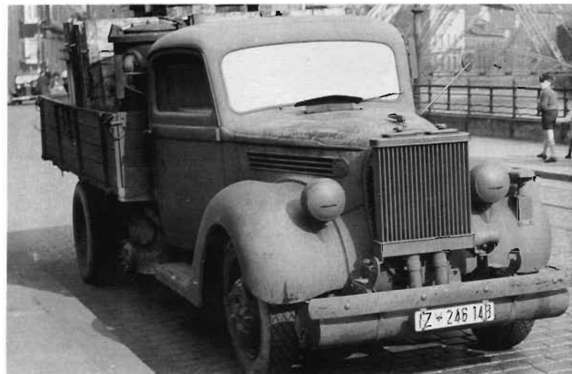
All Ford trucks could be modified to run on wood-gas for use back home. On the G 917 T (3.6-liter) and G 997 (3.9-liter) 8-cylinder types, the gas cooler (usually made by Imbert) was mounted in front of the radiator grille, the bars of which had to be cut off. On the G 987 T (3.2-liter) 4-cylinder type, the gas cooler was mounted under the motor hood. This picture shows a G 997 T in Wuppertal, with wood-gas system and Rhine Province registration with a "red chevron" (proof of permission for civilian vehicles). The gas generator (made by Imbert, 550 mm diameter) can be seen in the back, and under the bumper is the residue tank, the cleaning of which was an extremely unpleasant job.
