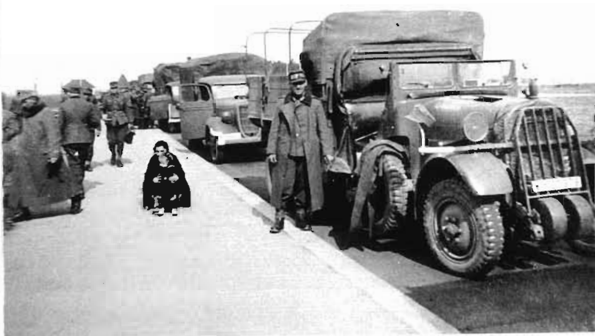
Vehicles of the 1st Mountain Division on the autobahn near Munich. In front is an Austro-Daimler ADGR (3 tons, 6 x 4, 72 HP), behind it a Ford V8-51.
