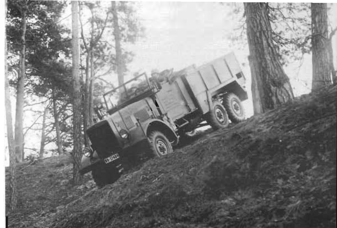
A factory-new "light off-road-capable truck, open, with uniform light truck chassis" on a test ride in 1938. The door lettering says: Net weight 4700 kg – Load limit 2425 kg or 25 persons – trailer limit 3500 kg – divide load evenly! (Photo: German Museum, Munich)
