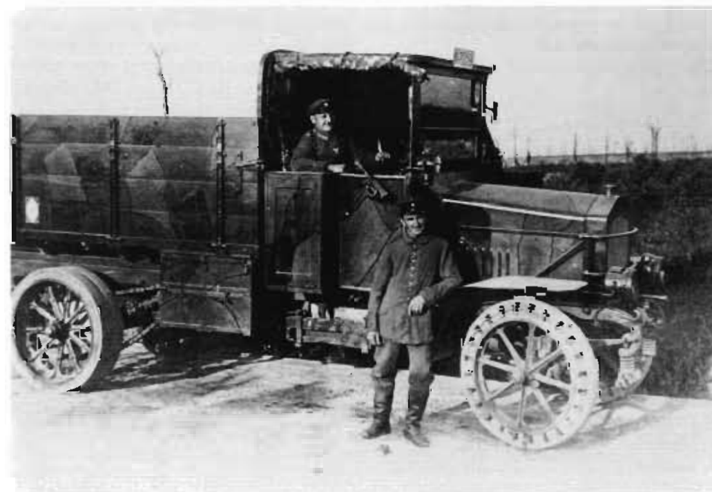
A 50 HP Hansa-Lloyd truck, first built in 1917 to carry a load of 3 to 4 tons. For lack of rubber (there was no Buna synthetic rubber then), the front wheels are fitted with sprung railroad tires. This bone-shaking makeshift solution required additional springs and chain drive instead of a driveshaft.
