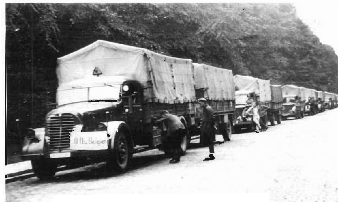
A truck column of the Organization Todt on the march to Belgium. In front is an "Österreichische-Automobil-Fabriks-AG" (ÖAF) ex-Austro-Fiat 5-ton Type FD6 with 100 HP Diesel engine (MAN license). The lettering on the sign means "Chief Quartermaster Belgium."
