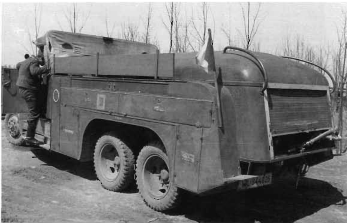
Two views of an "aviation fuel tank truck (Kfz. 384) with chassis of the medium off-road truck (o)", a Mercedes-Benz Type LG 3000 of J.G. 2, in northern France in 1942. Note the location of the exhaust pipe under the front bumper, customary for tank trucks, the slit cover of the main headlight, and the tires with the fairly uncommon "Wehrmacht tread." The tank had a capacity of 3500 liters of fuel.
