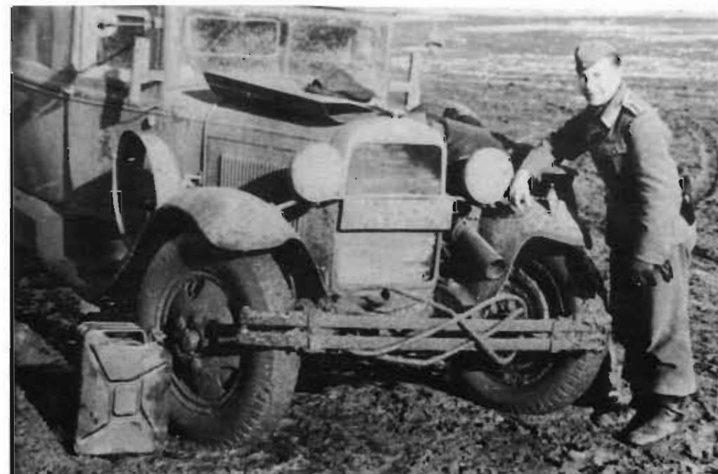
More than 9000 of the GAZ-AA were built with ambulance bodies. Here a captured vehicle (with camouflage) has just been cured of motor trouble. The type designation was GAZ-55 (at least for post-1942 models).
