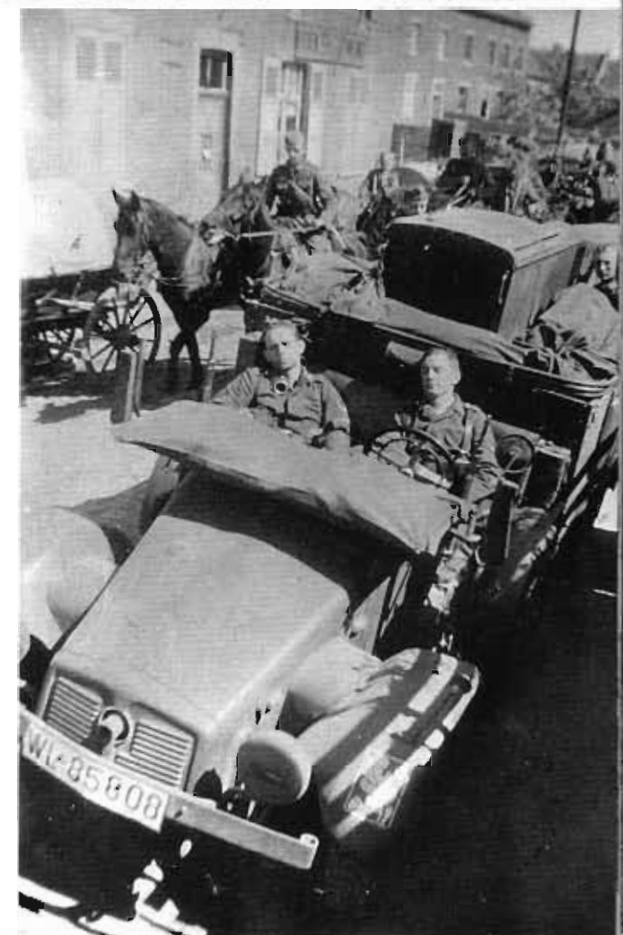
The Krupp L 2 H 143 personnel truck (Kfz. 70) of MG Battalion 6 of Coburg. The truck in front features several technical differences from the others: higher winch and spotlight mounts, different direction-indicator attachment, added wind deflectors and greater distance between the windshield and motor hood.
