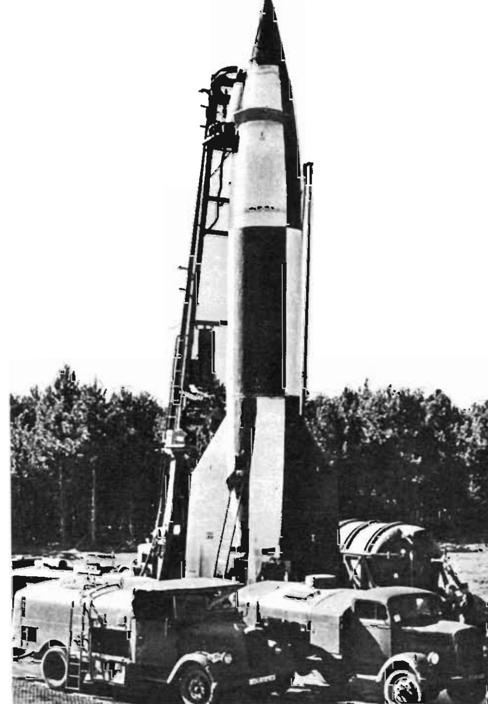
Peenemünde, Test Pad I, August 1, 1943: Preparations for the launch of an A 4 (V-2) long-distance rocket. According to "Procedure Instructions (secret), Special Vehicles, Components and Essential Parts of Ground Facilities FR (no date)", the trucks and trailers of rocket batteries were not given Kfz., Sd.Kfz. or Ah. numbers, but rather "Fahrzeug-Pos." numbers. The rocket stands on the "Launching Platform (Fz.-Pos.-Nr. 103), erected by "F.R. Trailer (s) (3-axle)(Fz.-Pos.-Nr. 102)", with "A-Stoff Trailer 6 (2-axle)(Fz.-Pos.-Nr. 402)" behind it, pulled by a Hanomag SS 100. At the left front is an Opel Blitz 3-ton Type S with open cab (customary for tankers) as "Tank Truck 3500 I B-Stoff (Fz.-Pos.-Nr. 404), at right an Opel Blitz 3-ton Type A as "Tank Truck 2100 I T-Stoff (Fz.-Pos.-Nr. 405)."
