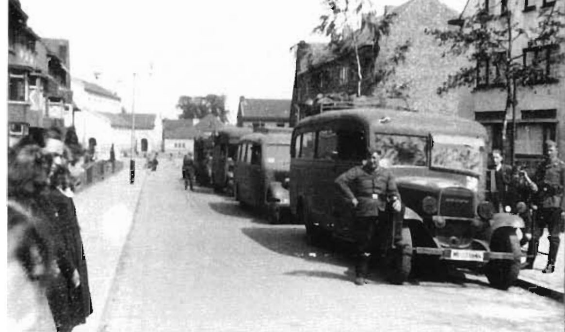
The sturdy chassis of the Opel Blitz was very well suited to use with bus bodies. This Luftwaffe bus used the chassis of the 2.5-ton Opel Blitz of 1935.
