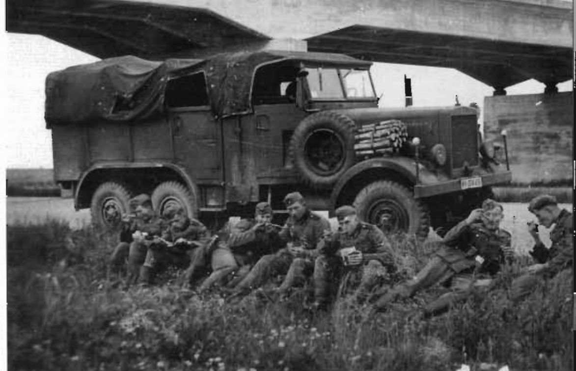
The "Survey and Equipment Truck (Kfz. 63" with uniform chassis for light trucks" was intended for a crew of 7 men plus driver and had an additional door to the rear area.
