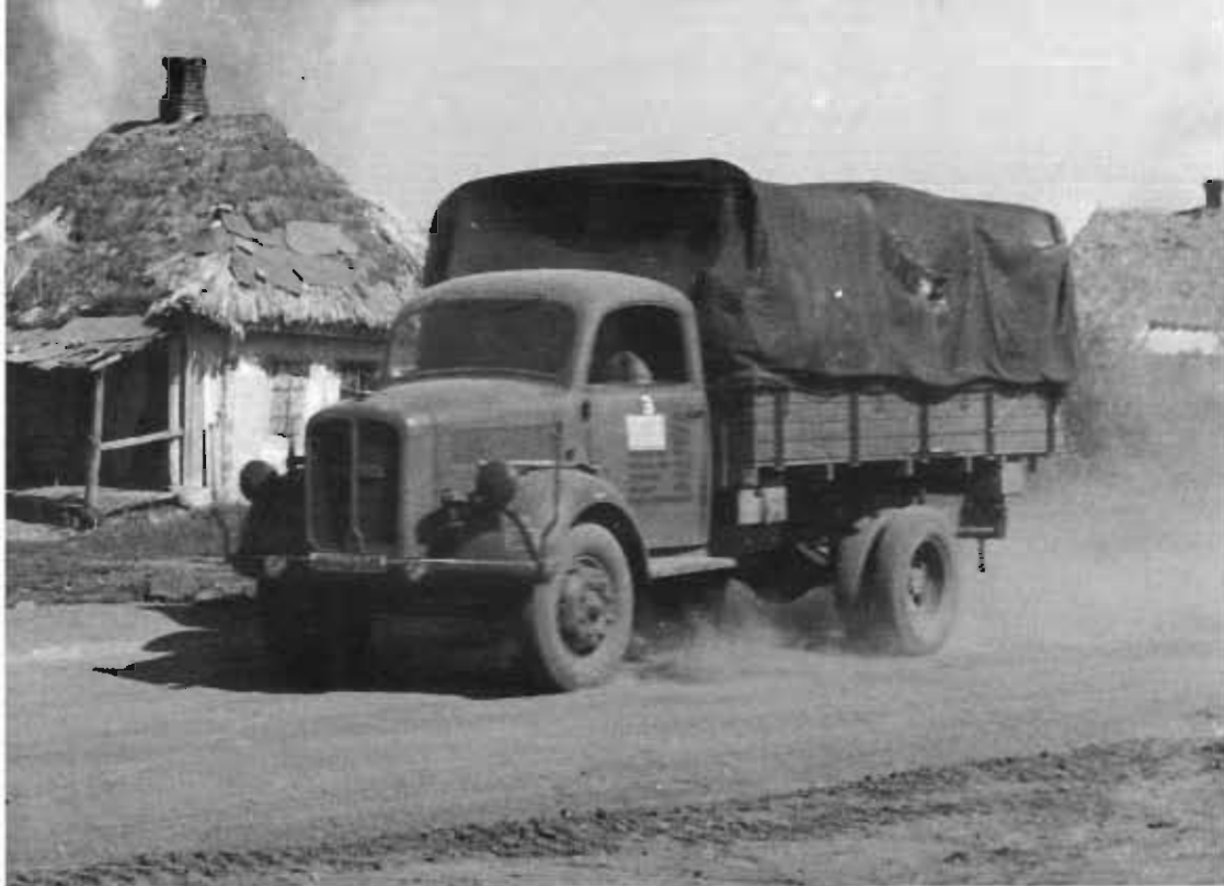
The further development of the Type G.W. was the "Lkw 3 t Borgward Type B 3000", which existed in A and S versions, and with 75 HP Diesel and 78 HP gasoline motors as of 1942. This picture shows a Borgward B 3000 S/D in southern Russia in the autumn of 1943. (BA)
