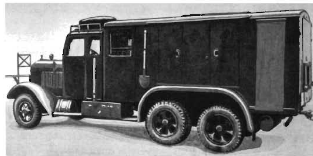
Personnel detoxifying truck (Kfz. 92b), in which contaminated personnel could get a thorough cleaning with warm water and chemicals.
