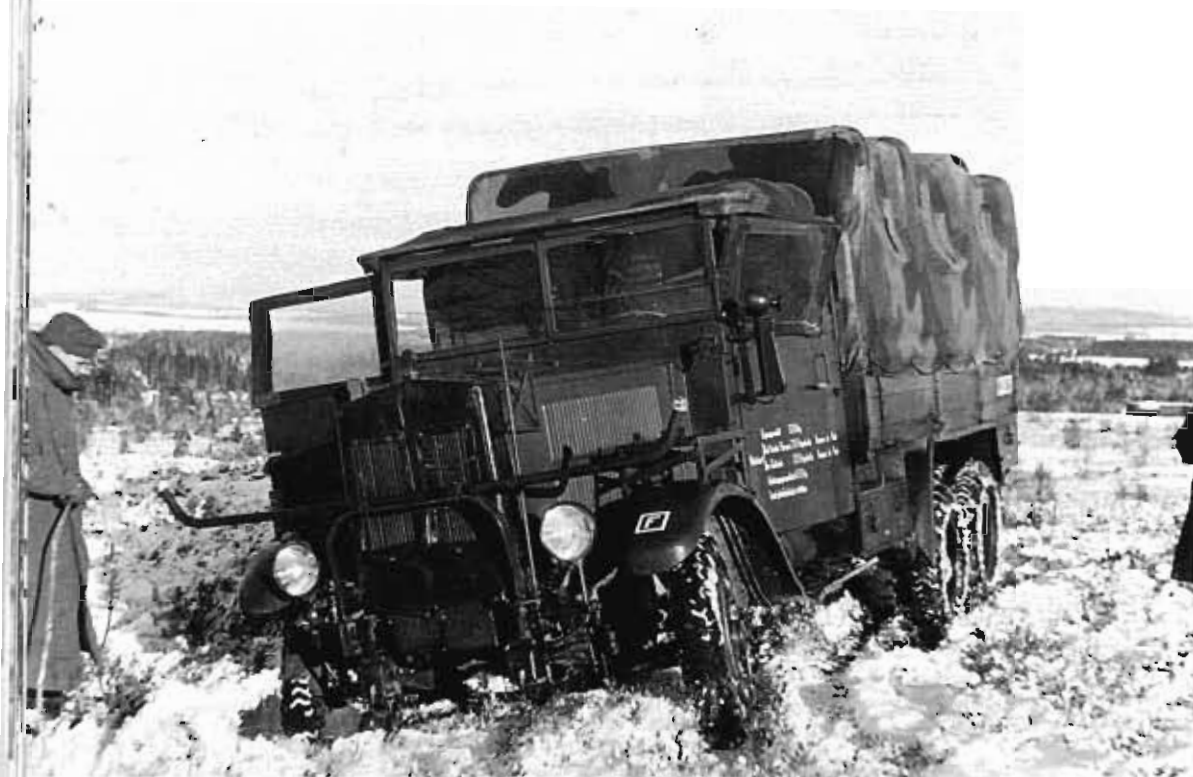
A Krupp L 3 H 163 at the Grafenwöhr driving school in March 1937. Note the Krupp name on the grille, the "antlers" ahead of the grille, and the telephone-cable racks on the fenders. The "F" shows it to be a telephone truck.
