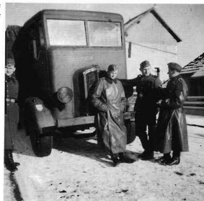
The Polish Polski Fiat 621 L (Fiat license) was built since 1931, with 12,600 built in all. The 4 x 2 vehicle had a load limit of 2.5 to 3 tons and a 50 HP motor. Photos of its use by the Wehrmacht, as here, are comparatively rare.
