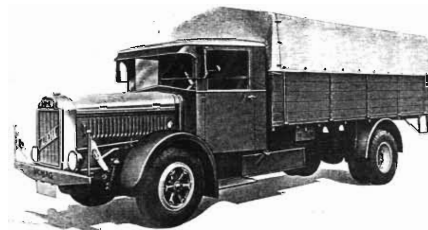
Vomag 5-ton Type 5L truck, Vomag 4 R 3080 with Diesel engine, 4 cylinders, 9.5 liters, 100 HP.
