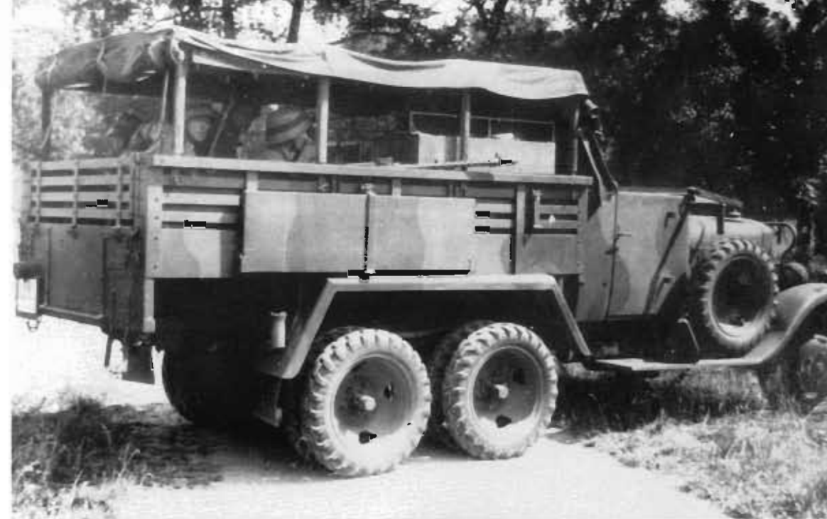
The light off-road (o) Mercedes-Benz Type G 3 a (6 x 4) was built from 1929 to 1935 and had a 6-cylinder, 3.7-liter gasoline motor producing 68 HP. This picture shows a personnel truck (Kfz. 70) of the Engineer Completion Company of Ingolstadt during maneuvers on the Ammer in Upper Bavaria in 1936, still bearing a Reichswehr number.
