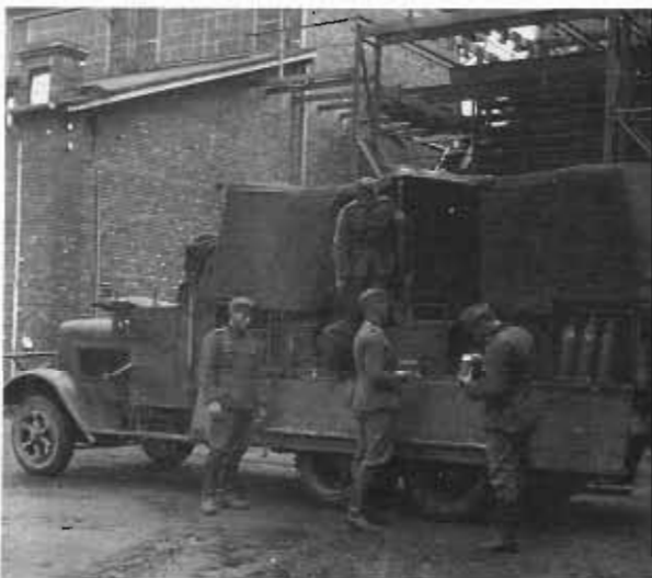
A Bridge Column B on the Autobahn: Henschel Type 33 as Engineer Truck 1 with Pontoon Truck (Pf. 11). The MG 34 gun, carried according to plan, is mounted on turning AA struts. Most trucks used by the grenadier and engineer companies were equipped with a "bottom hole for attaching the mount" in the bed, to be covered by a flap.
