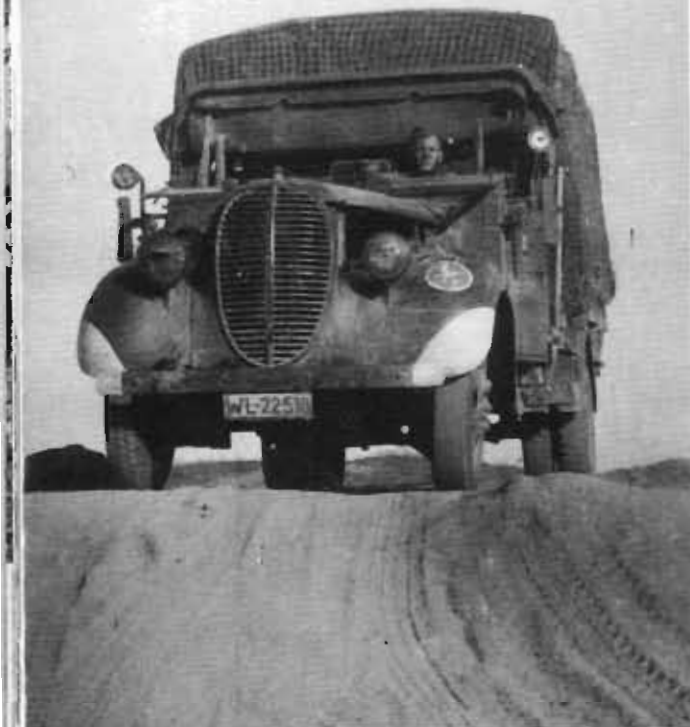
This type, with its oval grille, was made in the USA since 1938 and produced in somewhat changed form in Germany since 1939. The typical feature of all Fords made in Germany was the undivided front bumper. The 3-ton truck had a 3.6-liter Ford V8 motor giving 90 HP (Type G 917 T St IIIa) or a 95 HP, 3.9-liter Ford V8 as G 997 T St IIIb. (BA)
