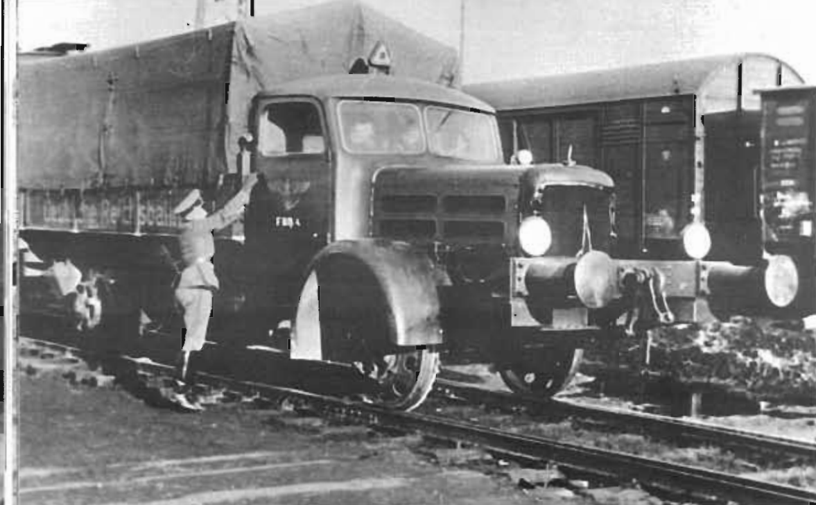
In 1941, forty Magirus L 365 6-ton trucks (with Deutz Diesel engines, 6 cylinders, 13.5 liters, 145 HP) were rebuilt into rail trucks at the Reichsbahn works in Opladen.
