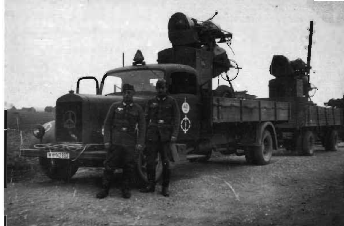
Mercedes-Benz Type L 3750 (WH-142 893) of an unknown unit (probably construction engineers) with building materials and cement mixers on the way to the West Wall. Road trains with two trailers, as seen here, reached a considerable length and caused a definite danger for the rest of the traffic, despite the warning triangle sign atop the cab. The L 3750 had a 6-cylinder, 7.2-liter, 100 HP Diesel engine and is easily recognizable by the Trilux front wheels.
