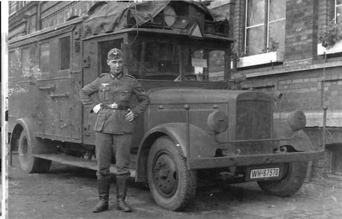
The 3-ton Magirus Type M 30 (4 x 2) was built from 1931 to 1934 and had a 6-cylinder, 4.5-liter gasoline motor giving 70 HP. The picture shows an intelligence workshop truck of a unit from Bremen in the spring of 1940.
