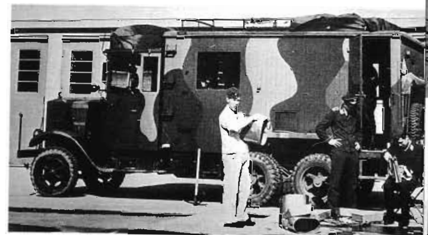
The Krupp L 3 H 63 as Flamethrower Truck I (Kfz. 74) with the chassis of the medium off-road Lkw (o). The truck was designed for driver, aide, and 12-man crew. Unlike the 163 version, Type 63 had louvers instead of vent flaps on the motor hood.
