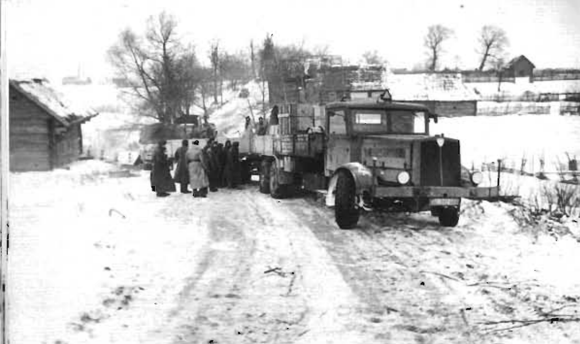
Winter 1942-43: Near Staranya-Russa this FAUN L 900 (WL-282684) laboriously crawls up an icy slope, pulling a trailer. The vehicle had a load limit of nine tons and could be driven by 6- or 8-cylinder Deutz Diesel engines with 13.5 liters and 150 HP or 18 liters and 200 HP.
