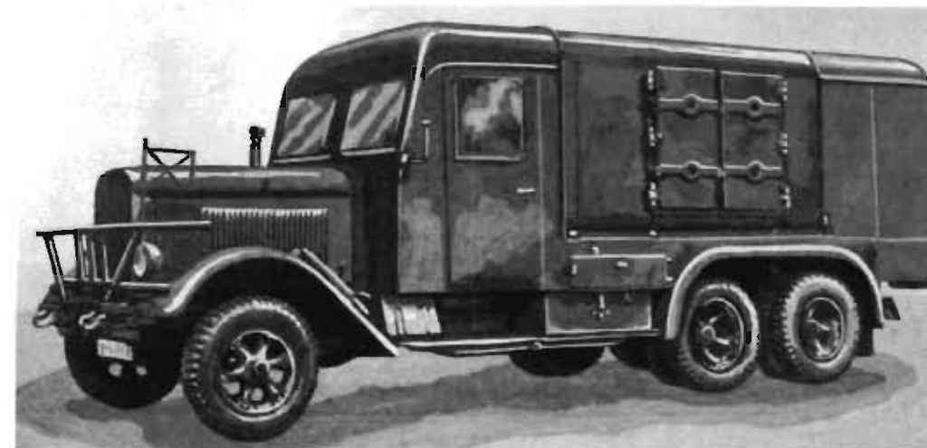
Clothing detoxifying truck (Kfz. 93), in which clothing could be cleaned of combat substances with steam and chemicals.
