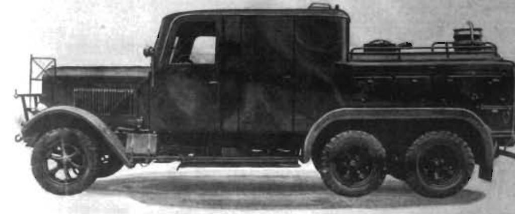
The trucks shown on this page were all special vehicles of the foglaying troops, on the chassis of the Henschel Type 33. They were rarely seen and usually used for other purposes. This picture shows a water tank truck (Kfz. 94). The vehicle could carry 2700 liters of water that could be warmed by a built-in heater and pumped to the detoxifying jets.
