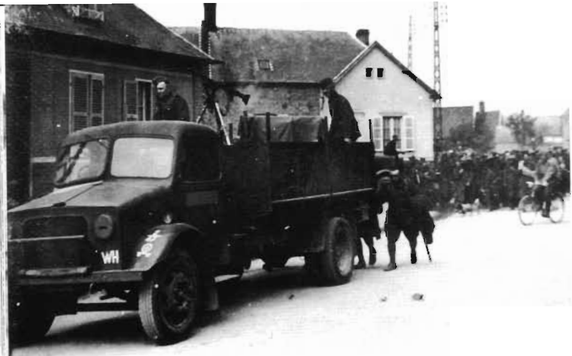
The Bedford OYD (4 x 2, 72 HP) was Britain's most often-built 3-ton truck (72,000 were built). The picture shows an early model (with dual rear wheels) with an MG 34 on a Tripod 34, guarding Belgian prisoners. The photo comes from an album of N.A. 27.
