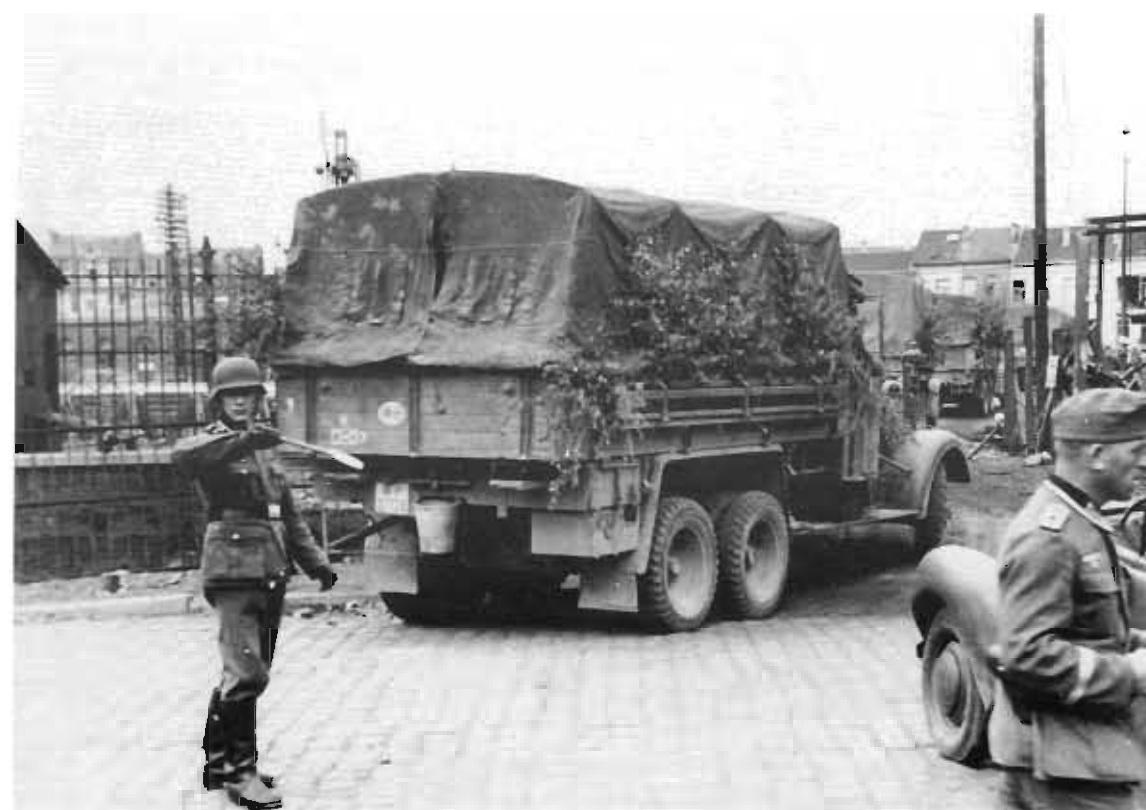
A very rare vehicle in the Wehrmacht was the Büssing-NAG Type KD (6 x 4), 415 of which were built for export to Turkey from 1936 to 1938. The vehicle had a Büssing-NAG LD6 Diesel motor that produced 100 HP. The grille guard and the pierced bumper were typical of it. This vehicle belonged to the 1st Mountain Division.
