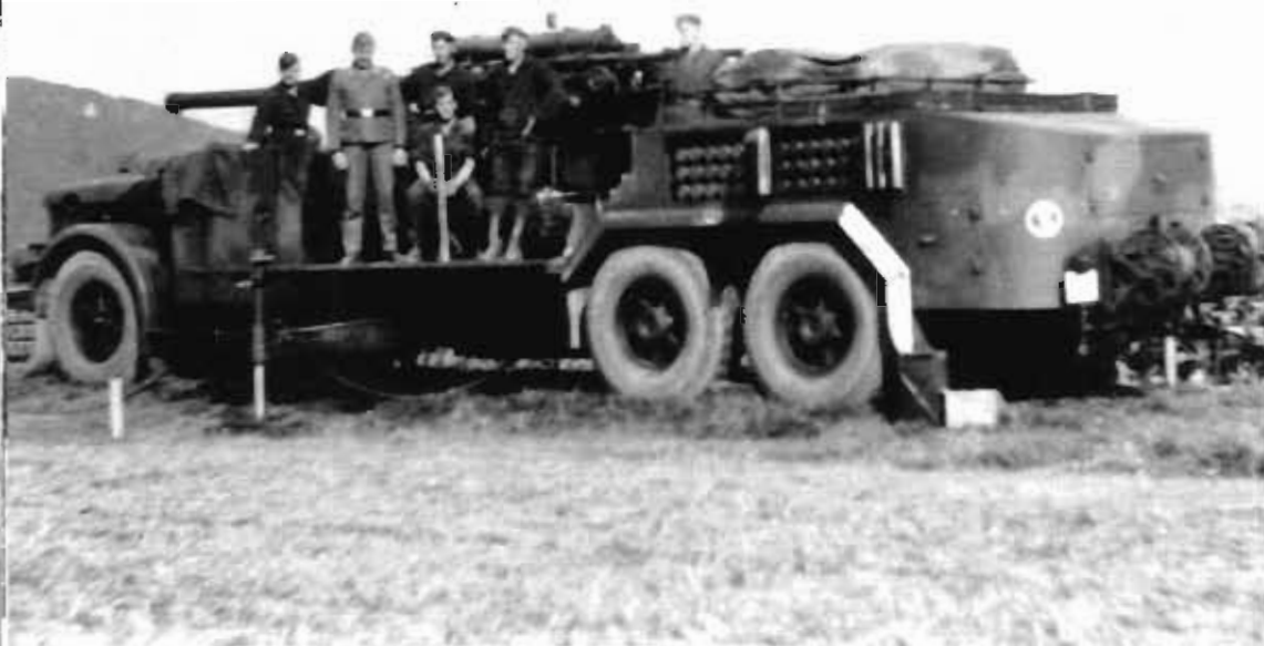
In the 1st Unit of Flak Regiment 42 (mot. S.), about 20 examples of an interesting vehicle came into being: the Vomag 9-ton low-floor truck (with bus chassis), used as a gun, survey or command equipment truck. This picture shows a gun truck with 8.8 cm Flak gun near Magdeburg in July 1941.
