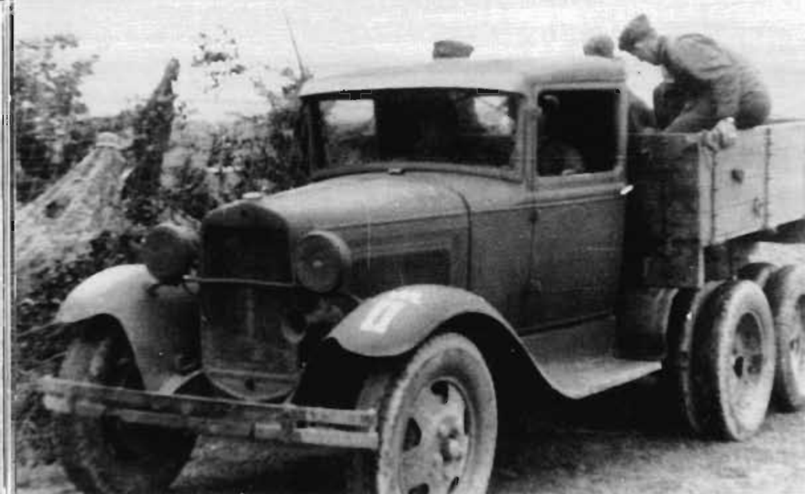
This GAZ-AAA was used by the 2nd Group of Fighter Squadron 3, as the Roman numeral II under the "WL" shows. The three-axle Russian Ford differed from the two-axle type only in having an additional axle and a somewhat more powerful motor; otherwise it was built exactly the same, and all parts were interchangeable.
