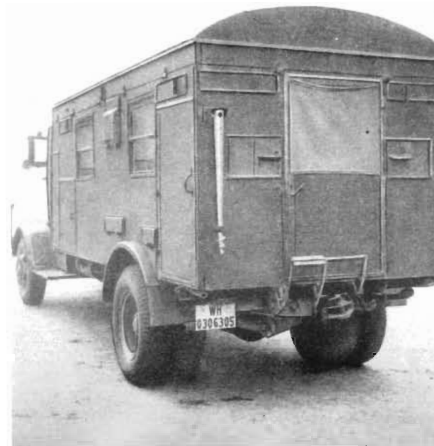
A Büssing-NAG Type 500 S with an additional opening in the rear body, as was seen, for example, in commissary trucks.
