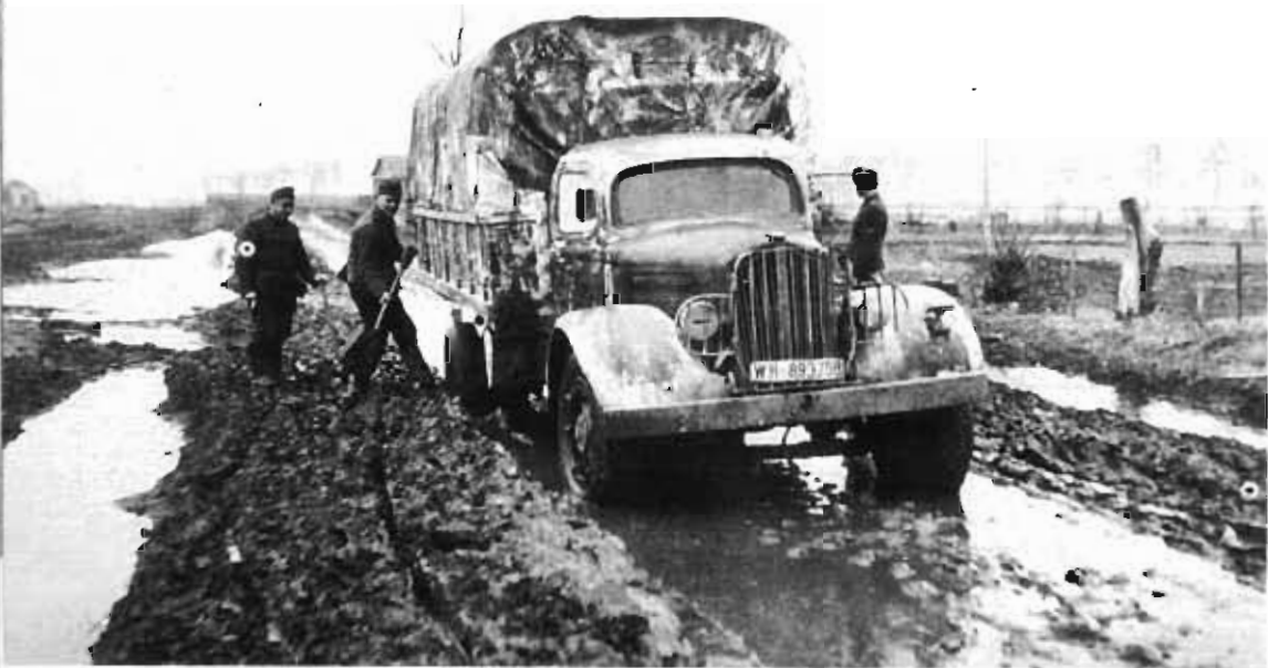
By the spring of 1940 the French Army had bought 1500 White 704 S (3 tons, 4 x 2, 85 HP) trucks from the USA. Large numbers of these outstanding trucks were captured by the Wehrmacht and naturally put to use. Infantry Regiment 51 had at least 15 Whites, which gave loyal service at Staraya Russa. The pictures show WH-893 758 and WH-841 853.
