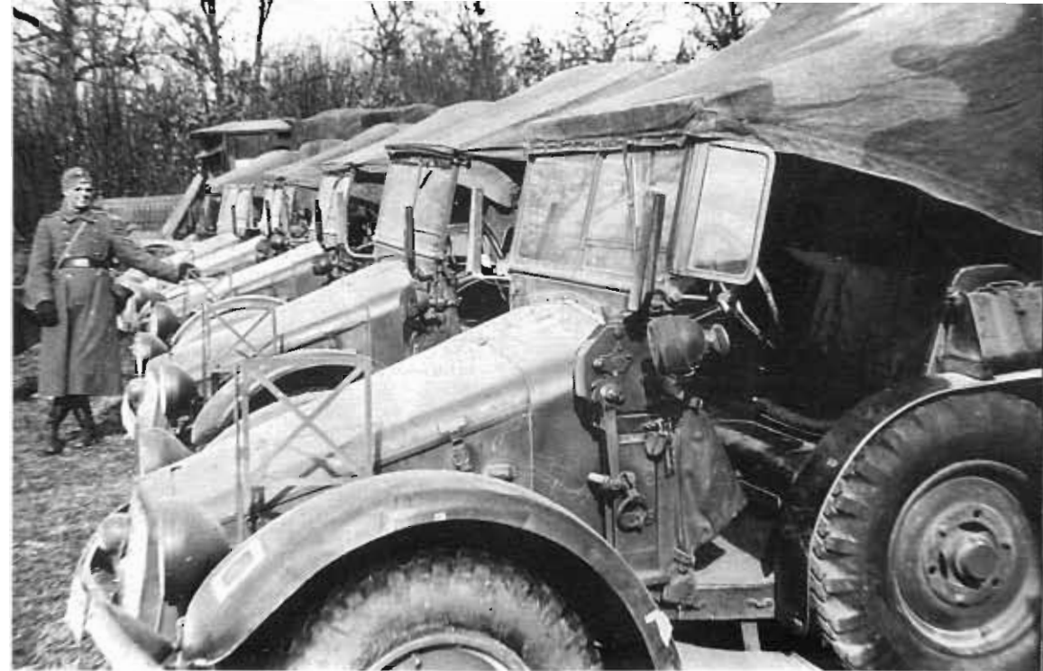
The Krupp L 2 H 143 personnel truck (Kfz. 70) of MG Battalion 6 of Coburg. The truck in front features several technical differences from the others: higher winch and spotlight mounts, different direction-indicator attachment, added wind deflectors and greater distance between the windshield and motor hood.
